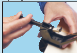
Step 5: Align the fibre
