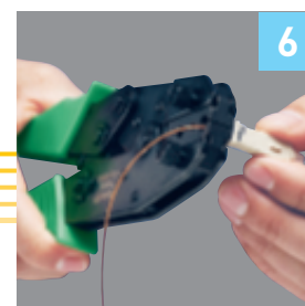
Crimp the fibre
