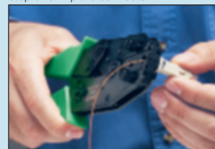
Step 6: Crimp the connector
