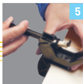
Align the fibre
