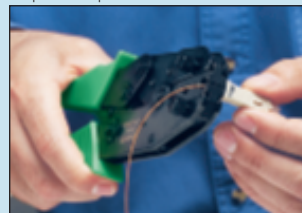
Step 6: Crimp the connector
