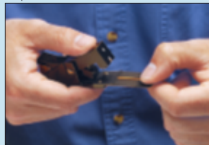
Step 5: Align the fibre
