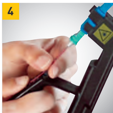
Insert the fibre in the connector
