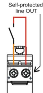
Or via a push button through the phase line protected by a circuit breaker on terminal C1
