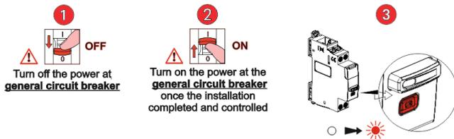
. 3/ Press and hold the Module Control settings button for more than 3 seconds, OR in the center of the General Scenario Wireless Command until the LED turns green, then release the button.
