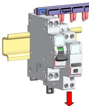
3. Pull the device downward in order to completely release it from the prongs of the busbar
