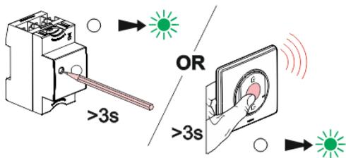
. The configuration LEDs of " with Netatmo " devices in the installation must all light up in fixed green.
