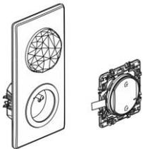
. 2/ Beforehand, the general circuit breaker must be turned OFF, and only after wiring step done, can be powered back ON to simultaneously power devices and allow them to be connected to the network.
