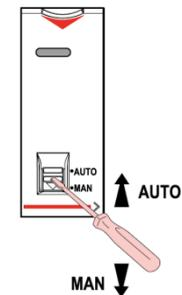
**Note:** in case of on-site maintenance, to put the selector on MAN is not enough. The use of a padlock is the only secured way
