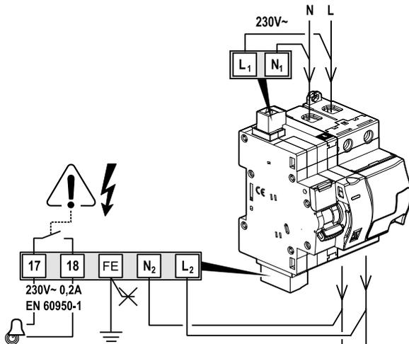
**Note:** It is not necessary to install a specific protection upstream of the Stop&Go because it is self-protected
