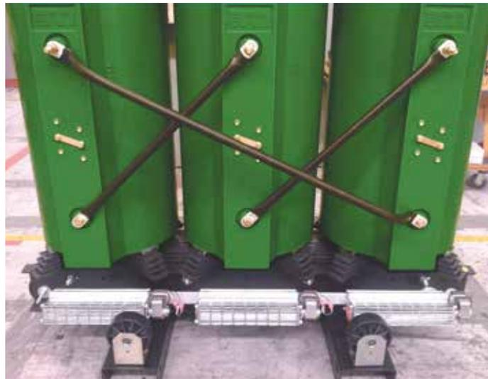
Example of transformer with ventilation bars
